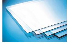
Applications must make adequate allowance for thermal movement, nominally 3.5 mm per metre. Adequate clearance must be allowed in the holes drilled for fixing. Sheet lengths have to be limited so that there is no excessive movement at the ends.
